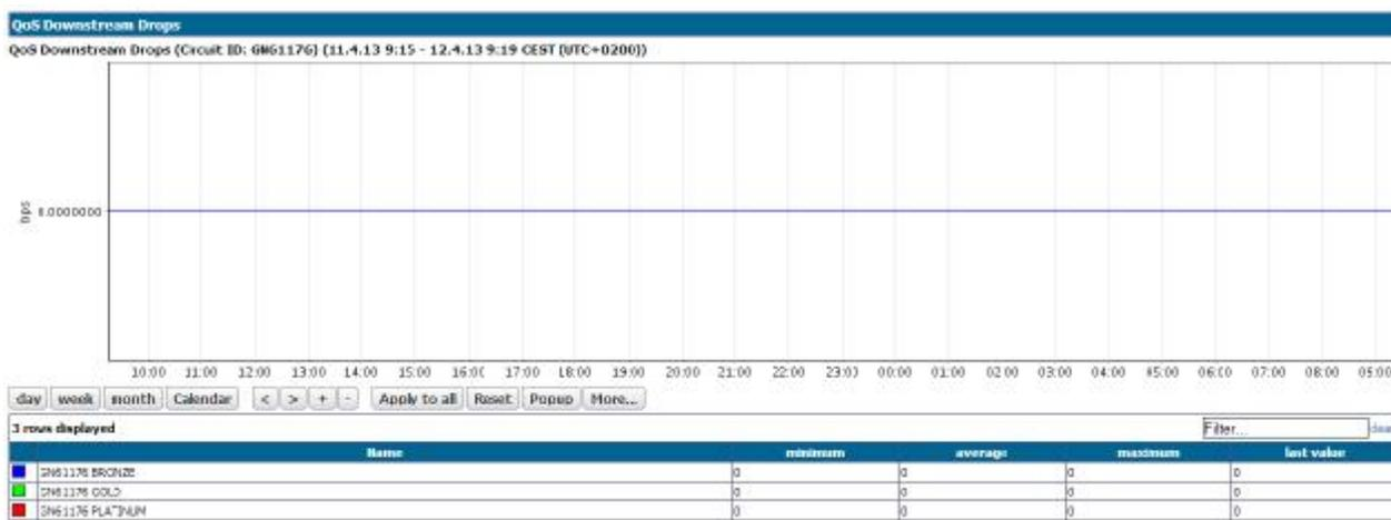
The graph shows the operations which did not fit within the framework of the QoS classes configured in individual classes and had to be dropped.
