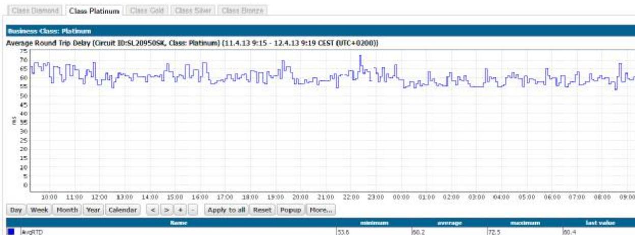
The graph shows the average delay of packets within the selected QoS class.
